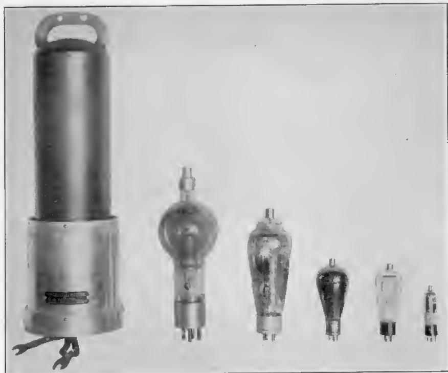
FIG. 52. A group of two-electrode, mercury-vapor-filled tubes. The average current rating, in amperes, of these tubes is: (from left to right) 100A., 12.5A., 6.4A., 2.5A., 0.5A., 0.125A.
